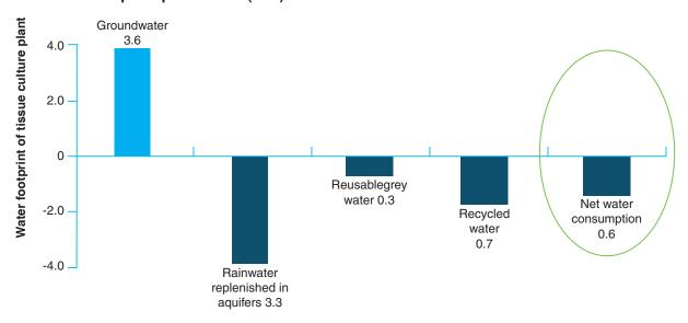
Through rainwater harvesting, 24% more water than the consumption was replenished into ground in 2017. Moreover the water used for irrigation of plants in polyhouses is recycled through a channel of pipes and filters. Thus, each plantlet produced in TC Park its net water positive.
